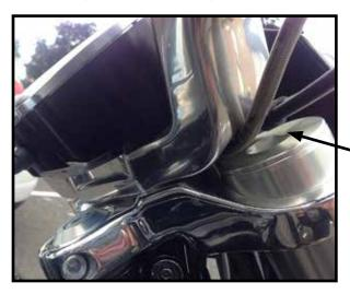
Note the factory location of the throttle cables and brake hoses.
